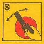
**SWEEP** from side to side... at the base of the fire until it appears to be out. Watch the fire area in case the fire flares back up.
