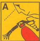
**AIM** low... pointing the extinguisher nozzle, horn or hose at the base of the fire.
