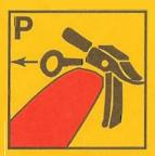
**PULL** the pin... Some extinguishers require releasing a lock latch.
