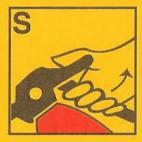
**SQUEEZE** the handle... this releases the extinguishing agent.
