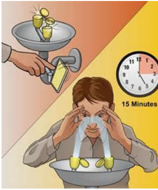
Figure 11.1 – Eye Wash Station
